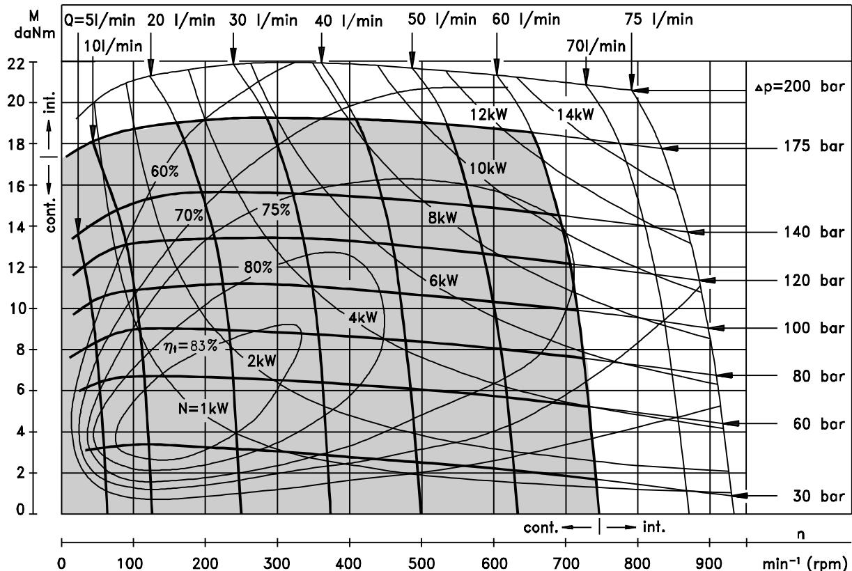
The function diagrams data was collected at back pressure  $5 \div 10 \text{ bar}$
