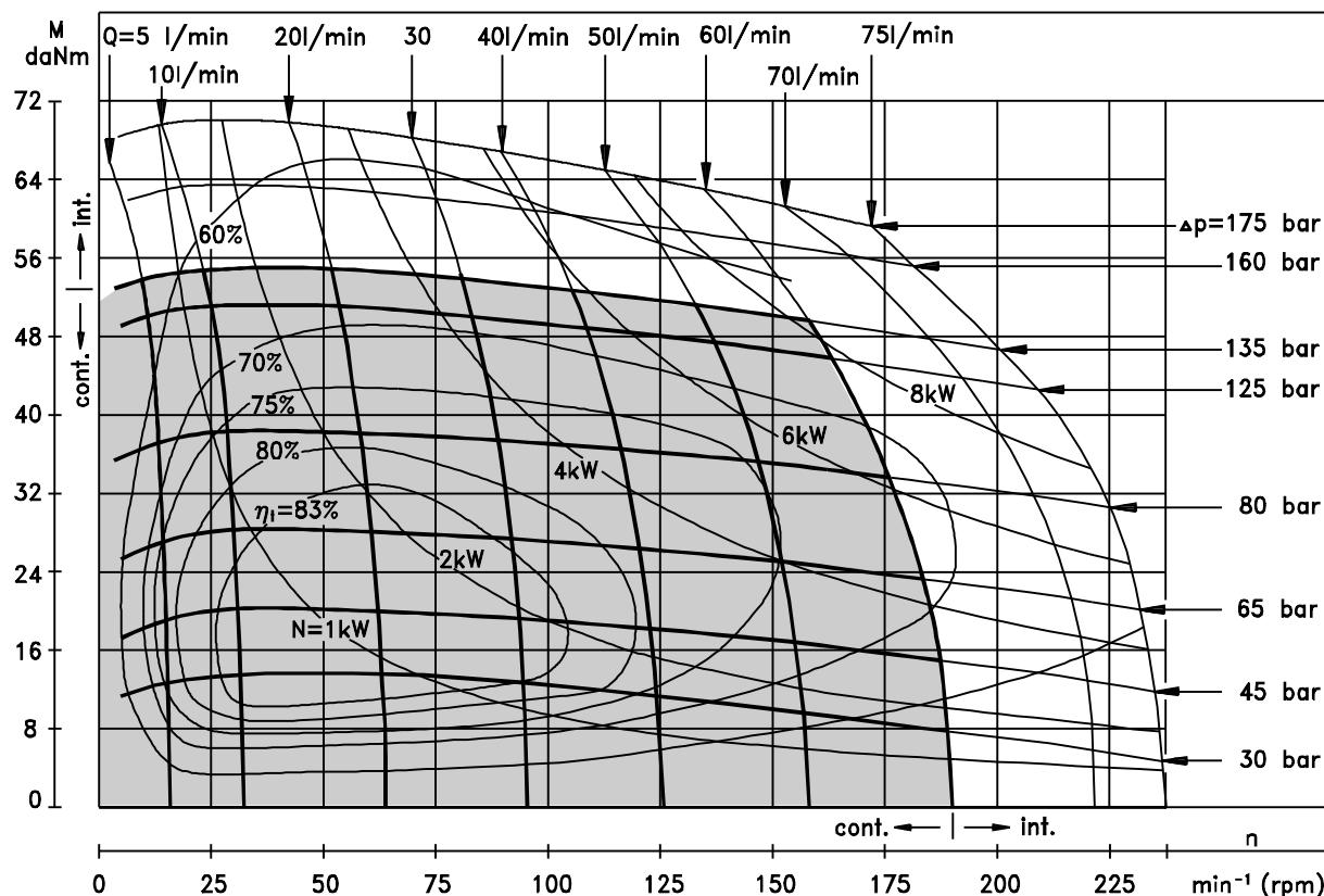
The function diagrams data was collected at back pressure 5÷10 bar
