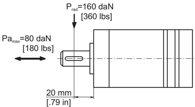
The permissible radial shaft load [Prad] is calculated from the distance [L] between the point of load application and the mounting surface:
