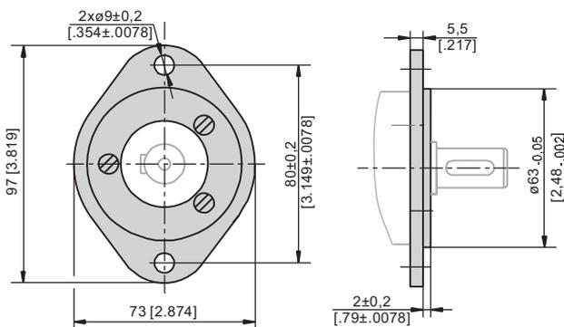
**F** Flange is mounted to the motor with 3 screws - M6x14. Tightening Torque: 5-6 Nm.
